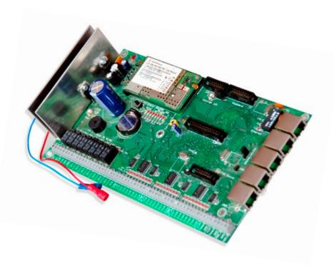
As a standard, the concentrator provides full functional interoperability with the Integra and Galaxy families of control panels from SATEL. It also acts as the concentrator for a group of the KP-2BS controllers within the Access Control System. After being supplemented with the IPS\_RS serial port module, the IPS concentrator can additionally monitor a fire alarm system control panel, using the Telsap 2000 or PMC 400 protocols.
